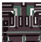
Topography of microchip, scan size is 70 x 46 µm
